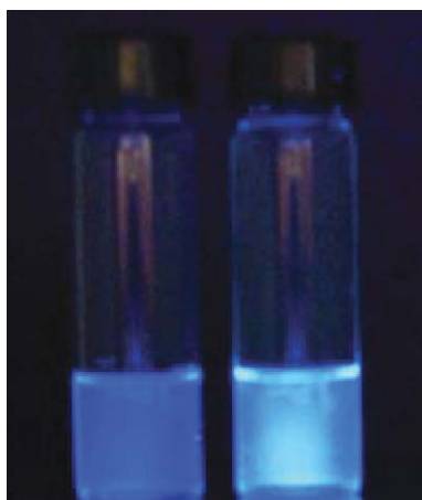
Fig. 4 The “naked eye” detection of triphosgene. Left: coumarins 1 and 2 in \text{CHCl}_3 before addition of triphosgene. Right: after addition of \sim 5 equiv. of triphosgene. The experiments were performed at 10^{-3} M, and the solutions were then diluted to 10^{-6} M. Both vials are irradiated at \lambda = 365 nm with a laboratory UV lamp.
